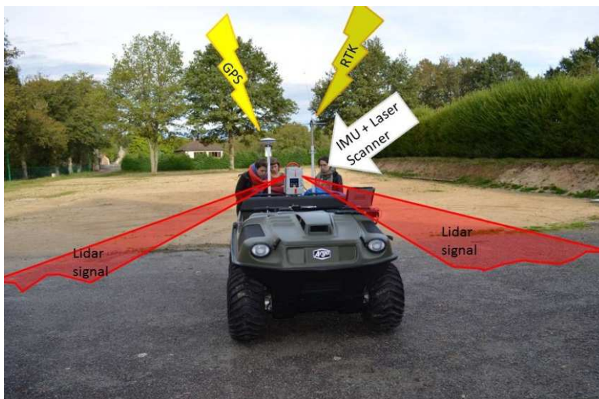
Figure 5. Main components of a mobile laser scanning system, mounted on the ARGO
